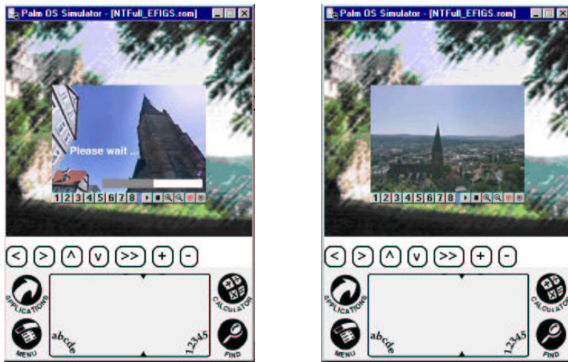
Figure 1: PTViewerME running in Palm Emulator: Displaying progress bar during JPEG-decoding ( left ) and displaying rendered view ( right ). A background image covers unused portions of the screen. The actual screen image is clearer than it appears in this PDF-document.
